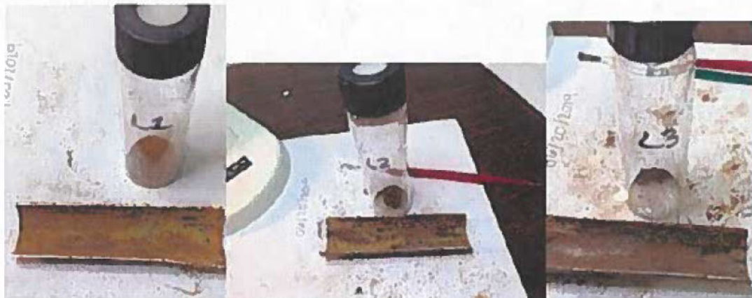
Figure 4-13 Layers of Scale Removed from Harvested Pipe
