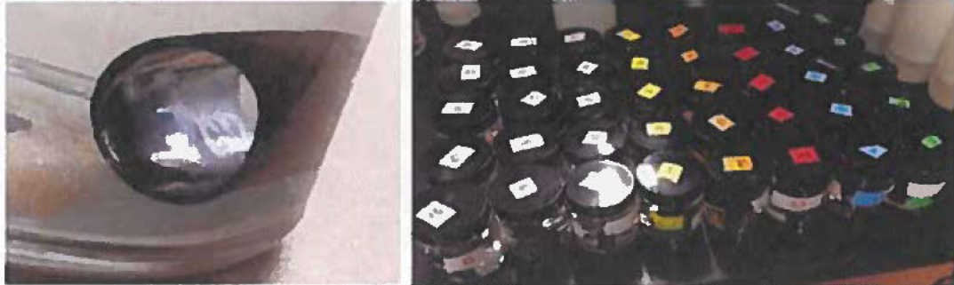
Figure 4-21 Apparatus Used for Testing. Solder Coupons in Glass Jars (Left) and 5 Replicates for Each Inhibitor Condition (Right)
